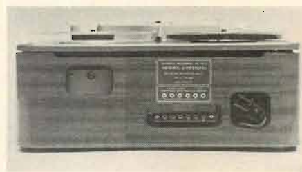
Fig. 3. Rear panel of recorder indicates line voltage to which set, and provides for the outputs and the high-level input. Small compartment at right holds power card.
